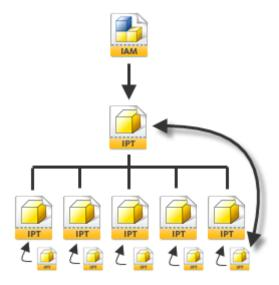
Unlike Multi-Body design, this method will add the Master part to the assembly and also constrain it and make it invisible. This component will already be set up as a Reference component structure.
