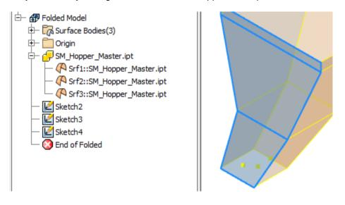
4. On the *Sheet Metal Tab*, start the **Face** command. Select one of the profiles created by the sketches. Make sure the geometry for the Face command creates the geometry to the outside of the surface loft since our design intent modeled the inside extents of the Hopper. Repeat for the remaining **2** sketches to create the **2** remaining faces.
