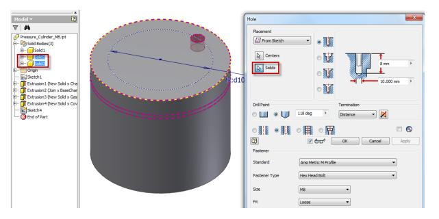
12. Create another Hole using the Concentric placement method. Use the top of the part as the Planar reference and the existing Hole1 as the Concentric reference. Create a Tapped hole using ANSI Metric M Profile, Size 8, Designation M8x1.25, Full Depth, and Right Hand Thread. Make the distance of the blind tap 30 mm. Be sure this time to deselect Solid3 and select only Solid1. You can use the Shift key to deselect solids.
