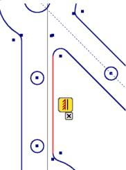
5. Place an Instance of the Sketch Block "**Centerlink**" next. Place this on the lower right hole in the Plate\_Web.
