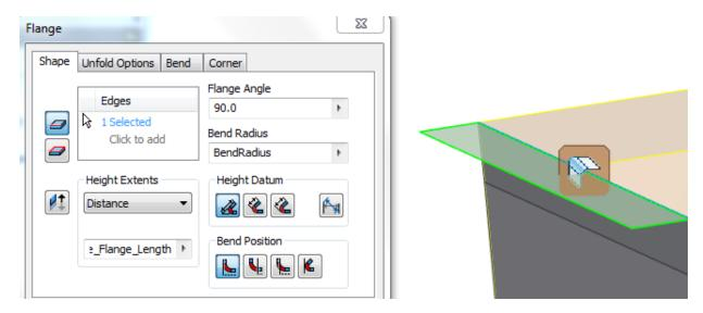
6. Start the **Sheet Metal Defaults** command (*Sheet Metal Tab > Setup Panel*) and uncheck the *Thickness from Rule* box and set the value equal to *Ga\_Thickness*.
