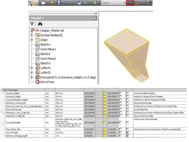
2. Close the Parameters dialog box and select each sketch in the Model tree examining the equations in the sketches. This geometry was modeled with surface lofts, but could just as easily be created with solid geometry. Close the file, do not save changes.
