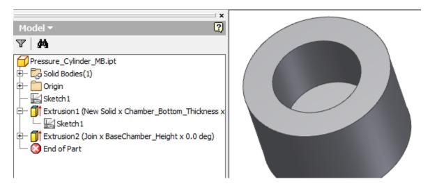
6. Create a new 2D Sketch on the top face of the part. Notice the edges of the cylinder are automatically projected. If they are not, use Project Geometry from the *Draw Panel* and select the two circular edges. Finish the Sketch.
