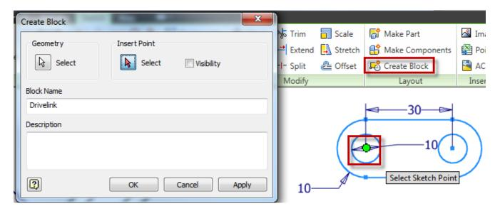
10. Apply **Coincident** constraints to the **Drivelink** and **Rockerlink** circle center points as well as the **Drivelink** and **Plate\_Web** circle center points. Make sure no other constraints get created that restrict movement. If this does get created, make sure you delete it.
