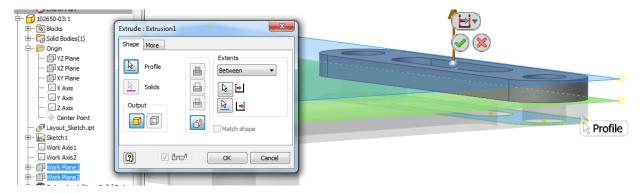
You can also create Pins for the links using middle-out design with in place components. (Make sure if you do not want Adaptivity to hold down CRTL when projecting references)
