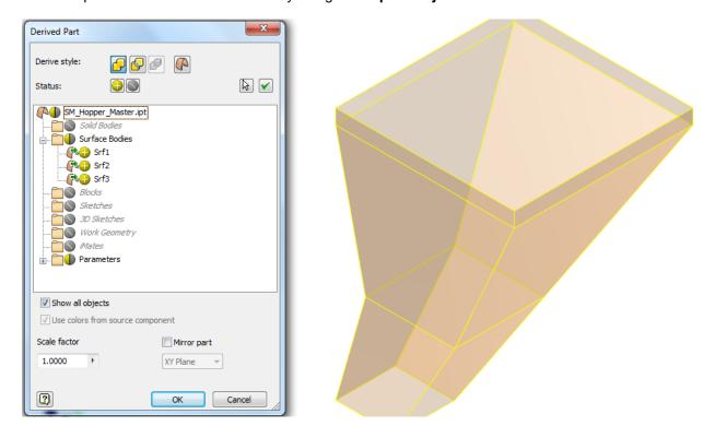
3. Create 3 new sketches on each of the highlighted faces. You may need to project the edges manually if *Auto-Project Edges* is turned off in the Application Options.
