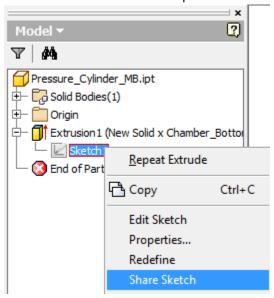
5. Choose **Extrude** again, this time selecting the outer most profile. Set this extents to *BaseChamber\_Height*. Make sure you are joining the material instead of cutting. When finished, turn off the Visibility of Sketch 1.
