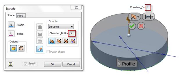
4. Expand Extrusion 1 and right click on Sketch 1 and choose the *Share Sketch* option. This will allow you to use the geometry in the sketch over and over again without having to create a new one for geometry that can be defined on the same plane.
