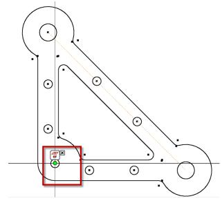
4. Place a Vertical Constraint on one of the vertical edges of the Sketch Block. This will lock the sketch block's position in the sketch.
