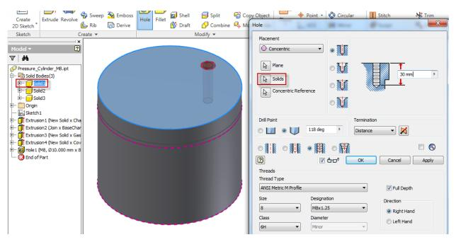
13. Since we did not set the value for the termination distance of the first hole, the connection does not go through the part all the way. Go back to **Hole1** and modify the depth of the hole to be equal to *Gasket\_Thickness + CoverPlate\_Thickness*.
