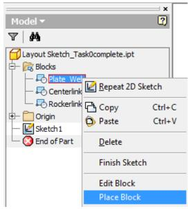
3. Place the Block's insertion point on the Origin of the Part file.
