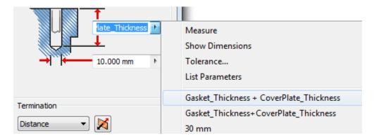
14. Also adjust Hole2's depth to be Hole\_Depth. These adjustments will allow the depth of the holes to be consistent with the Gasket and Cover Plate material thicknesses as well as maintain good thread engagement.
