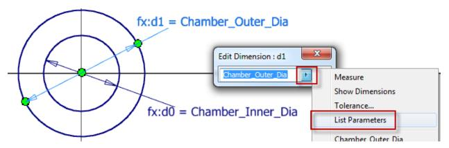
3. Finish the Sketch and **Extrude** by the Parameter *Chamber\_Bottom\_Thickness*. Remember to use the right arrow on the input boxes to get the *List Parameters* option to make sure the parameter name matches exactly.
