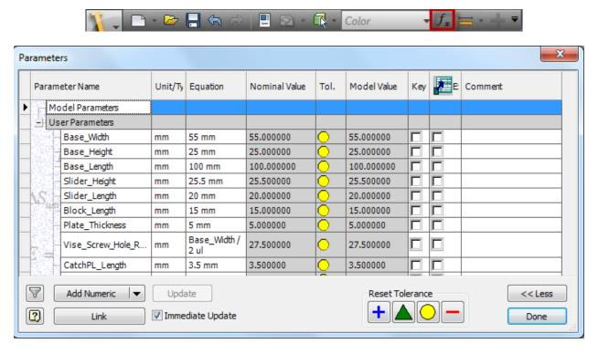
Parameters can be renamed and accessed without having to constantly open this dialog box. For instance when you see this icon in an Edit Dimension box or Feature Dialog box, you can list a named parameter to link to the modeling/sketch dimension.
