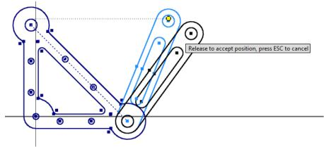
7. Place an instance of the **Rockerlink**, this time place it in space and do not attach it to anything. Place a **Coincident** Constraint between two of the circles on the links.
