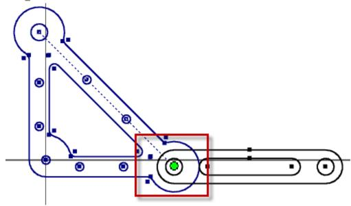
6. Click and hold on the **Centerlink**'s outermost center point and drag it around. Notice the **Centerlink** is constrained to the center point of the **Plate\_Web**'s circle.
