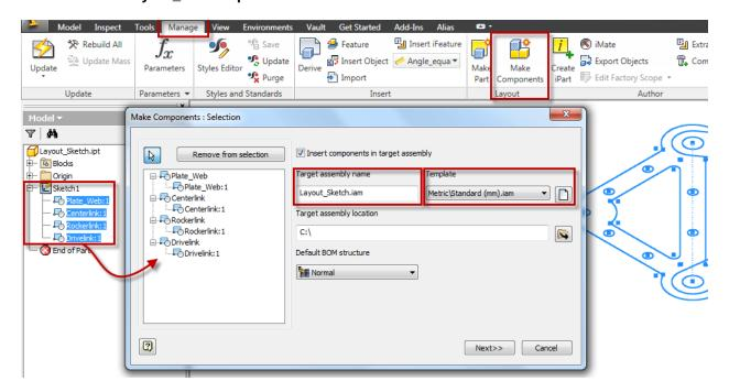
2. This next box will allow further setup of the files that are to be created from the Sketch Blocks. Template selection, overriding source directories, parameters, and constraint creation could all be done from this box as well as more unique file naming. Change the names of the files as shown below (102650-01, 102650-02, etc.) and also make sure they are using the **Standard** (mm).ipt template. Click Ok.
