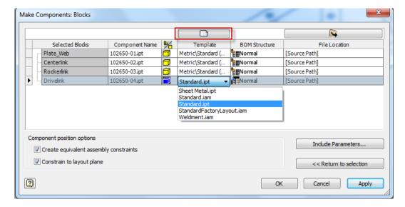
3. A new assembly file will be opened with the Layout\_Sketch.ipt file placed an Invisible component with a BOM structure set to Reference. Assembly constraints will be setup based on the sketch constraints used during the layout process. There will also be some assembly constraints suppressed based on this same reasoning.
