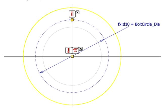
11. Create a Hole using the From Sketch placement method. Size a Clearance Hole for ANSI Metric M Profile, Hex Head Bolt, M8, Loose Fit. Make sure you use your Solids button highlighted below to include both Solid2 and Solid3 in the operation. Otherwise the Hole will only permeate through Solid3.
